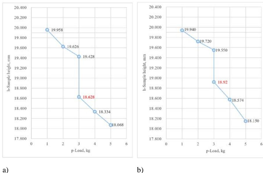
Figure 4: Dependence of change in sample height on load with soaking at 3 kg for soil ratio: a) without geotextile; and b) with geotextile.
