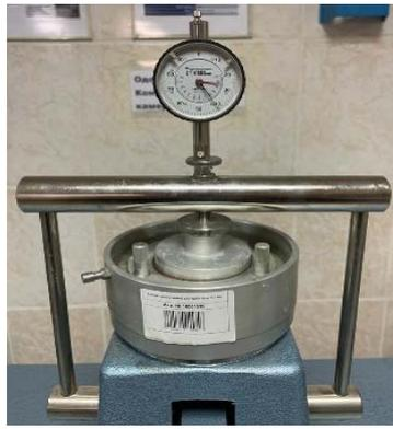
Figure 3: Testing of quasi-soil samples on a uniaxial compression apparatus.
